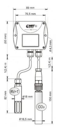
CO2 concentration, temperature and relative humidity t-line Web sensor. Remote alarm.
